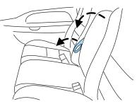
To gain access to the storage compartment in your armrest, lift the latch to open the lid. The lid cannot be opened in the upright position.
